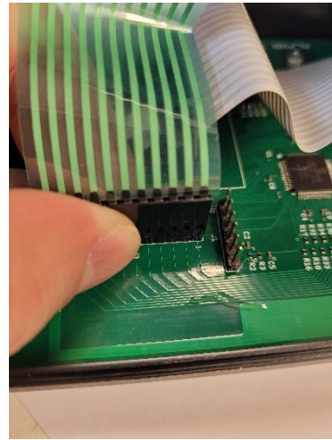
2. Firmly and slowly remove green ribbon cable.
