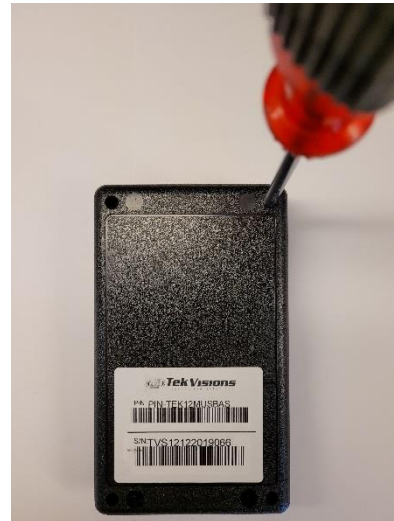
4. Replace 4 small Phillips screws. Reconnect ArmourScan and test.
